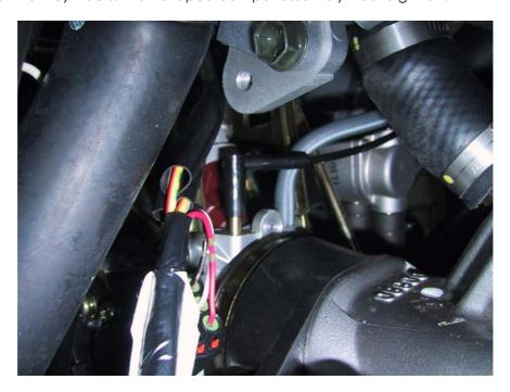
To fit the dispenser I made my own mounting plate which uses the paddock stand bobbin mounting bolt. I used a 45mm long bolt and fitted the plate with a nylock nut. A couple of P clips then keep the injector pointing in the right direction. Img\_0548
