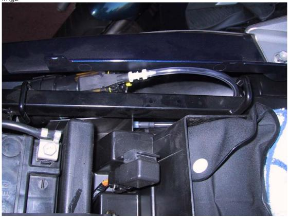
On the V-Strom you can use either the front or rear vacuum connection. Img3 shows using the front cylinder vacuum point which can be accessed looking up between the V of the 2 cylinders. The L shaped damper assembly fits straight on.
