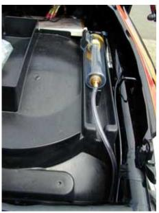
Dispenser position as shown, in the two pictures below. NB: Usual dispenser position is onto sprocket with 45degree cut facing outwards as per next picture.
