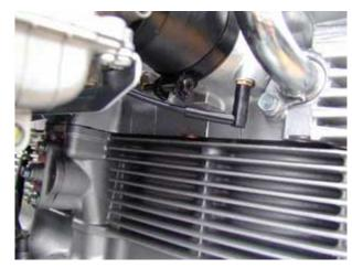
With the CB1300 attach the vacuum connection on the right side at the fourth cylinder, as shown in the photograph on the left.
