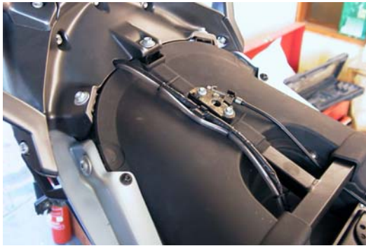
Route tubing as shown. We supply a piece of viton tubing, to protect our Scottolier tubing around the exhaust pipe. It's selected for its high temperature and oil/petrol resistance.
