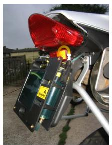
I also fixed an aluminium backing plate to the HCR itself and the lot was then assembled to the number plate holder to make the good stiff mounting, suffice to support the weight of the filled HCR.
