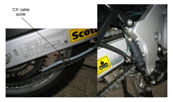
The dispenser head should be angled such that the slash cut dispenser is away from the sprocket and can drip oil onto the chain. If you turn it around it will pick up dirt off the sprocket & get blocked.
